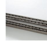
Substructure consists of layered cardboards (B-flute) for more stability and a high quality appearance
